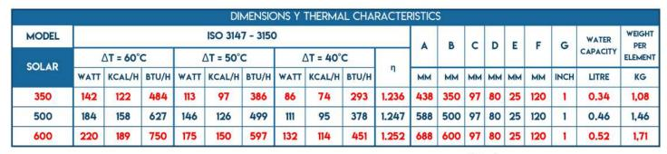
Output in Watt/hr a 60°C room temperature through tests according ISO 3147-3150.
